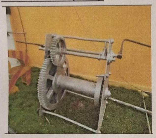
They work by either wind up or wind out a roof/ cable or adjusting the tension of the rope. They are used to recover vehicles raising sails, lifting elevators and snowboarding.
